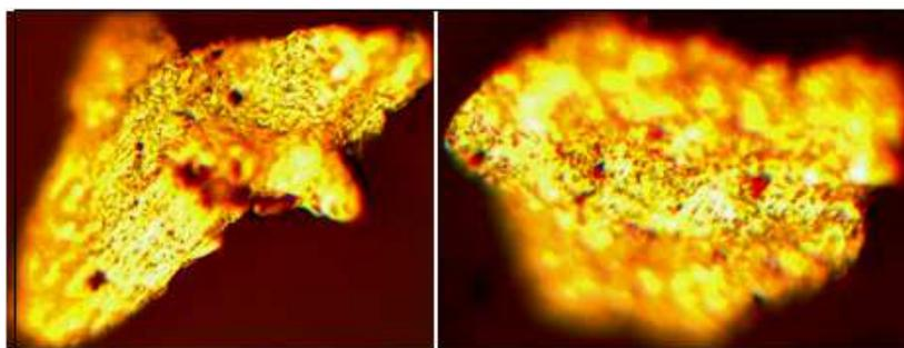
**Figure 9: High Alloy Steel Particles**
