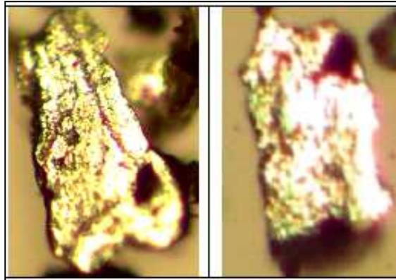
**Figure 5: Fatigue Wear Particles of Straight Edges**
