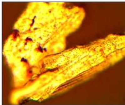
**Figure 8: High Alloy Steel Particles after Heating to 450 °C**
