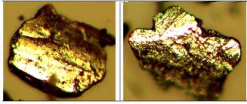
**Figure 4: Fatigue Wear Particles Retained by the Oil Filter that Disassembled from the Tested Combustion Engine**
