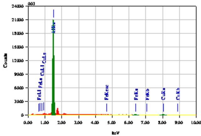
Figure 13: Quantitative Analysis of the Wear Particles and Solid Contaminants
