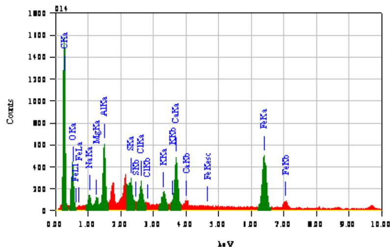
Figure 19: Quantitative Analysis of the Wear Particles and Solid Contaminants
