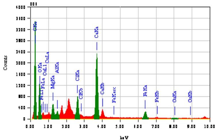
Figure 15: Quantitative Analysis of the Wear Particles and Solid Contaminants
