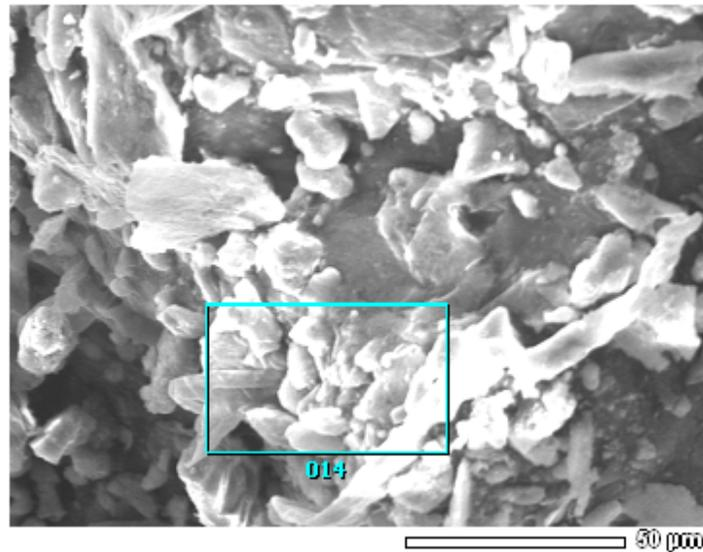
Figure 18: Scanning Electron Microscope of Wear Particle
