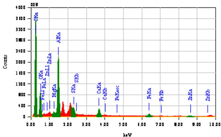
**Figure 17: Quantitative Analysis of the Wear Particles and Solid Contaminants**
