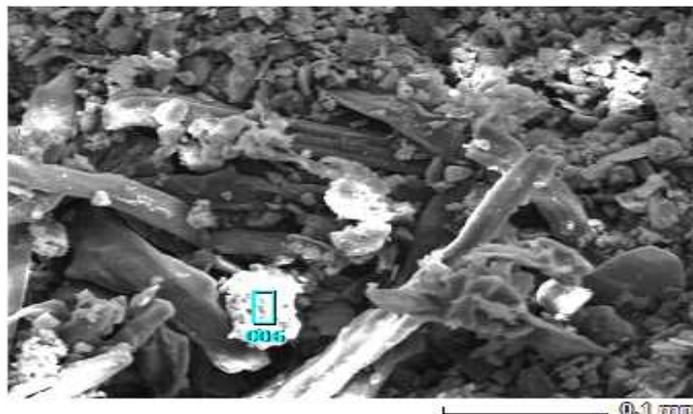
Figure 14: Scanning Electron Microscope of Wear Particle
