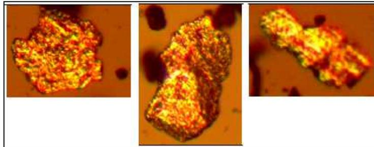
**Figure 11: High Alloy Steel Particles Heated Up to 540 °C**
